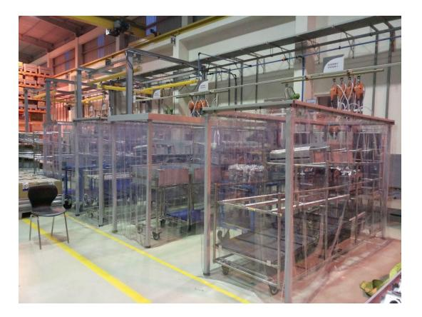
•Luke India needed a specific solution to protect their jigs and tools from dust settling on the same. This resulted in minimum cleaning and damage to the tools increasing productivity, accuracy and longevity.
