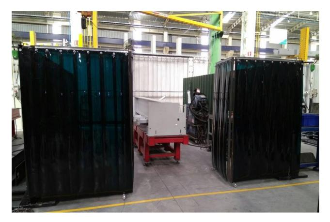
Sophisticated welding zone needs attention to details to ensure that the harm full rays / sparks / smoke and molten materiel do not escape to other areas which can cause serious damage to men and materiel around the work area.
